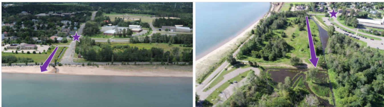
Pictures depict how the project rerouted storm drain discharge from Lake Superior (left) to wetland plantings (right), where it is filtered. Stars mark a common reference point, and arrows show the general direction of flow.
